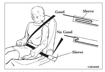
The lap belt portion of the front UNIBELT has a sleeve inside which the belt is folded back over itself in a loop. This allows the belt to help absorb the energy of a collision through a controlled release of the loop. In the event that the loop inside the sleeve has come loose, replace the entire seat belt assembly.
